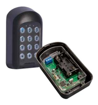
The CENTURION SMARTGUARD and SMARTGUARDair range provides efficient, secure keyless access control by enabling users to store up to 1000 unique codes comprising one to ten digits in its non-volatile memory. A variety of electrical devices can be activated (including gate operators, alarm panels, water pumps, etc.) by making use of one or more of the outputs provided.
